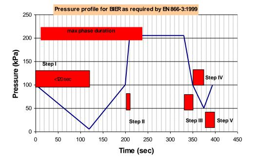
The pressure profile required by the standards (and defined here as "theoretical") can be used to calculate the temperature profile for an environment where saturated steam conditions are obtained.
