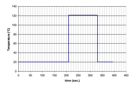
A BIER complying with the standard EN 866-3 (Biological systems for testing sterilizers and sterilization processes – Particular system for use in moist heat sterilization) as well as the ANSI/AAMI ST44:2002 (Resistometer used for characterizing the performance of biological and chemical indicators) must have the following performance:
