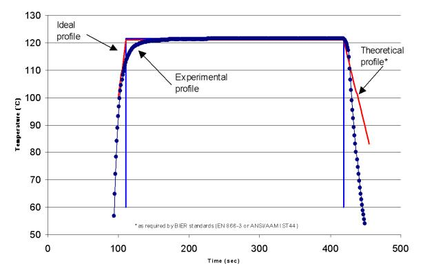
Another example of temperature profile relevant to a different stainless-steel test-tube with a volume of 2 ml is reported in the following picture.
